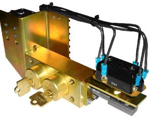
The Type SKRU consists of an interlock, a solenoid, and an auxiliary switch. The solenoid is designed to permit removal of the interlock key in response to an external electric signal. The auxiliary switch is a quick-make, quick-break device, which operates when the interlock key is rotated. Normally, the keys are trapped in the SKRU and the solenoid is de-energized. To release the keys, a signal must be sent to the solenoid from an external source.
